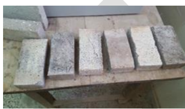
Figure- 7. Concrete specimens after 2 hrs. of high-elevated temperatures
