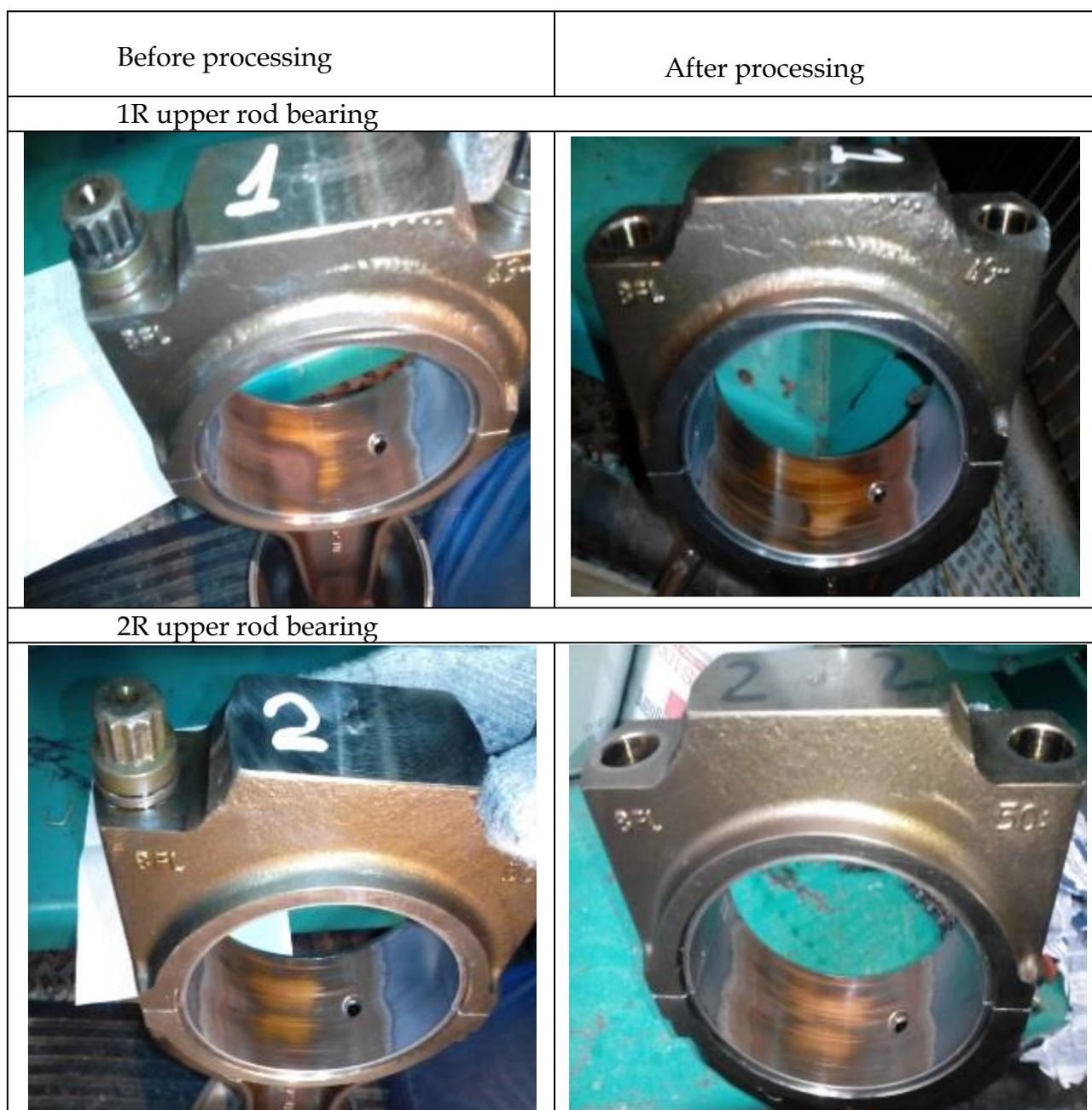
Figure 3. External view of bearings of rod journals
