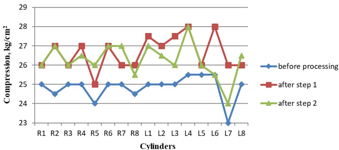
*Figure 4. Change in compression by cylinders*
