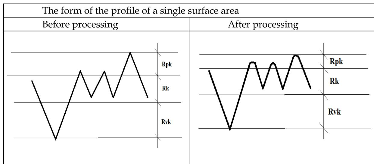
Figure 5. Changing form of the profile of a single section of a honed surface
