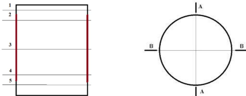
Figure 2. Scheme of measuring the inner diameter of the sleeves
